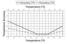
Figure 2. Temperature Accuracy
