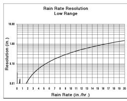
Figure 3. Low Range Rain Rate Resolution
