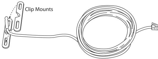
3. Position the clip mounts over two of the mounting posts on the closed plate. Make sure you orient the clip mounts as shown in the illustration below.
