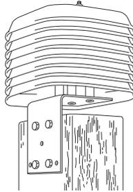
1. Using the power drill with 3/16" (4.7 mm) drill bit, drill three holes through one of the closed plates in the locations marked by small dimples on the bottom of the plate.
