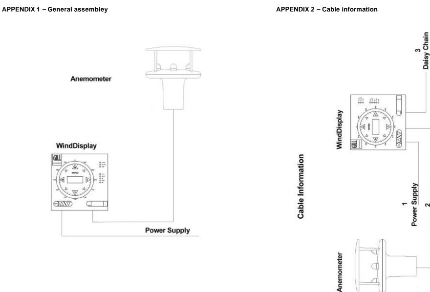
3 = 1 Twisted pair 7/0.2 RS422 compatible 2 = Twisted pairs RS422 compatible 7/0.2
